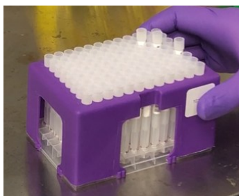
Figure 10 Lift the rack of 96 Mitra devices off its protective high wall microplate and plate the rack of devices over the microplate. Some devices may not immediately drop into the well. Touch these gently and they will drop into place, then push the rack of device so it is flush with the bench surface.
